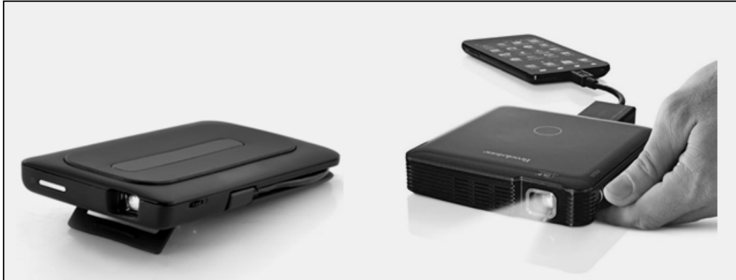
Figure 2.6: DLP Cell Phone Projector and DLP Handheld Projector
