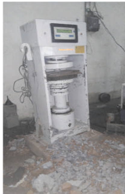
Photo Plate No. 5 Shows the measurement of concrete block strength of various foundry sand used.
