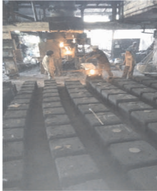
Photo Plate No.3 Shows molten ferrous material collection and pouring into sand molds.
