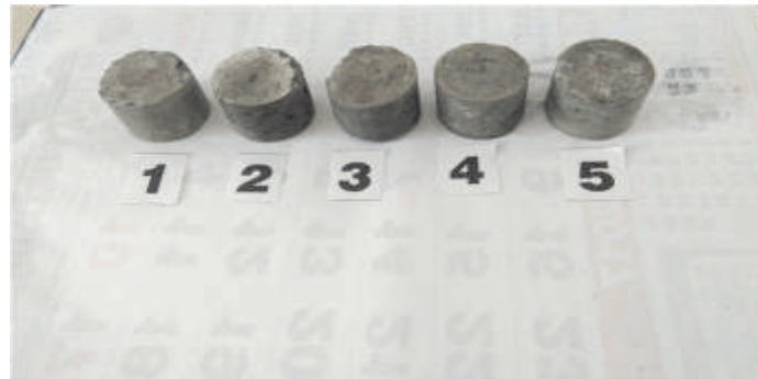
Photo Plate No.4 Shows concrete blocks processed from various foundry sands.
