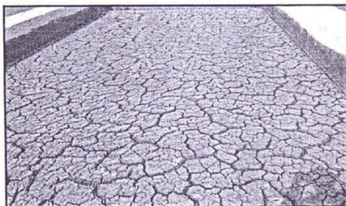
Photo plate 8 : Dry sludge cake generated from ETP.
